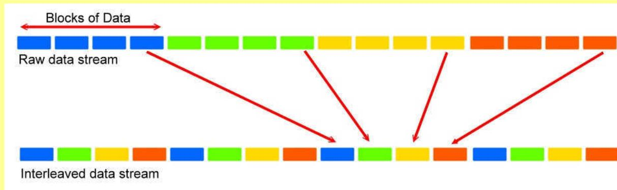
If your line is particularly susceptible to bursts of noise then interleaving should improve your VDSL2 experience simply because if you lose a whole batch of data then this could cause your bridge to loose sync with the exchange.
