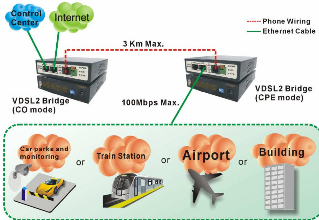
**Figure 2.6 VDSL2 Bridge point to point application diagram**
